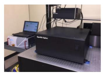
Sparkle Optics 200-W Illuminator Laser is a reliable turn-key computer controlled laser for long term operation
